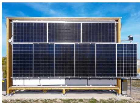
Outdoor test stand for facade integration
