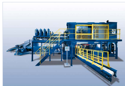
An MBM installation for recycling PET composites
